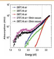
of electronic structure temperature, solution-processed indiumzinc-oxide thin-film transistors is probed, using X-ray photoelectron spectroscopy, ultraviolet photoemission spectroscopy, and photothermal deflection spectroscopy. A compensation of a significant density of acceptor states below the conduction band by shallow hydrogen and oxygen vacancy-induced donor levels is identified as the key factor for achieving high device performance at low temperature.
