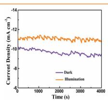
The cathodic current of a MoSe<sub>2</sub>-rGO/ PI composite film hardly decreases at -0.6 V compared to SCE by current density versus time curves, both illuminated and dark, illustrating how it possesses high stability and sufficient cathodic current density. These properties show its potential as a better catalyst for hydrogen evolution reaction, and even solar-driven hydrogen evolution.
